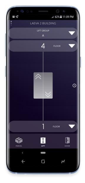
The simple interface offers the tenant's a choice of **LIFT GROUP** (bank of elevators) as well as movement between their allocated floors. After choosing the floors the tenant wishes to move from and to, a swipe of the slider in the direction of travel immediately places a call to the elevator system which dispatches the next available elevator.
